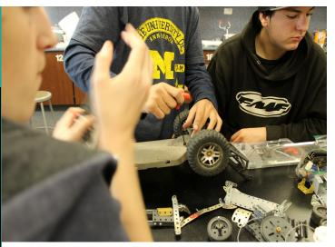
Karrie Magrini's *Electrical Engineering* students at Temecula Student Center have *decided to make a rover that will deliver a beverage to a person*. Students have made their first iteration of a prototype using a remote control car, transistors, PVC pipes, a servo motor, and other materials. Next, the students will *make their own rover* and learn what they need to make the rover move via *electrical circuits* and *computer programming*.
